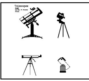
Amateur telescopes come in many sizes and shapes, but basically comprise two types, reflectors and refractors, in four categories. From top left, clockwise, a Newtonian reflector, a Schmitt-Cassegrain reflector, a Newtonian reflector on a Dobsonian mount, and a 60-mm refractor. A beginner's first piece of optical equipment, however, should be a pair of binoculars.
